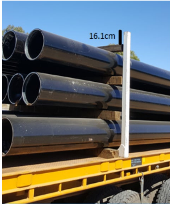
Image 1: Pipes, separating wood blocks and stanchions – note the top (fourth) row had been removed in this photograph
