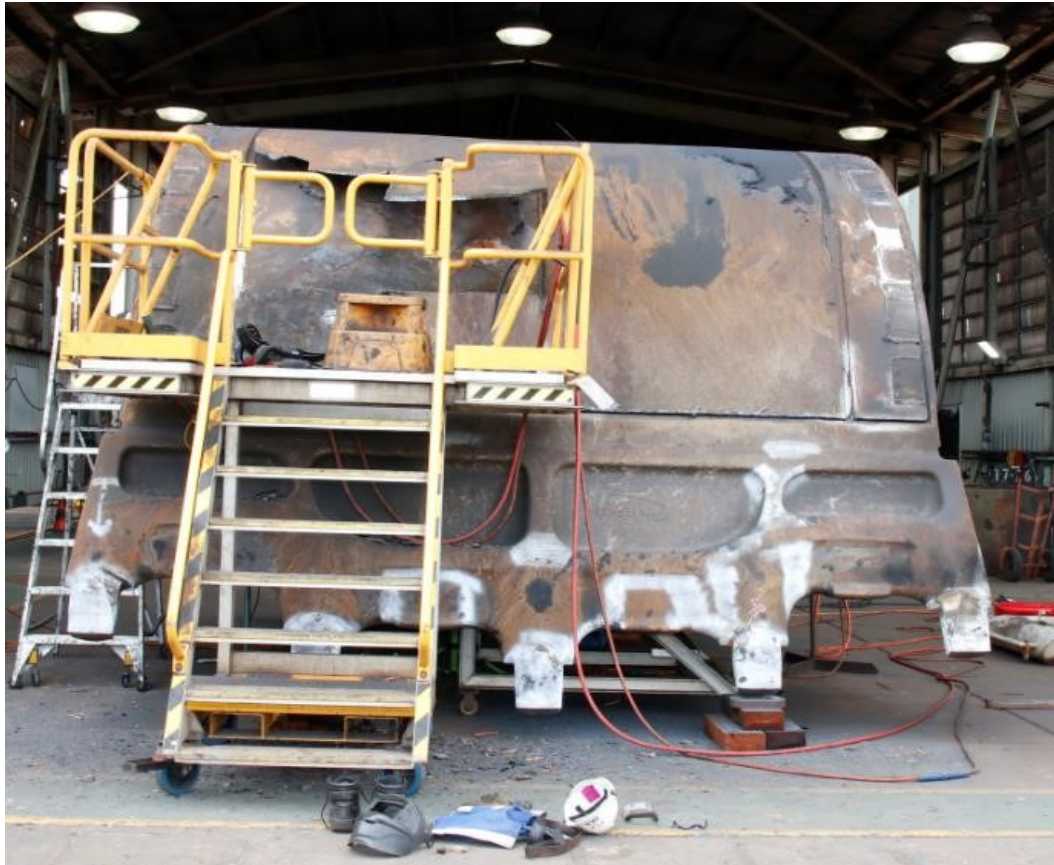
Photo of work platform in situ from which Mr Springer was working on bucket #1 at the time of the spring back event.
