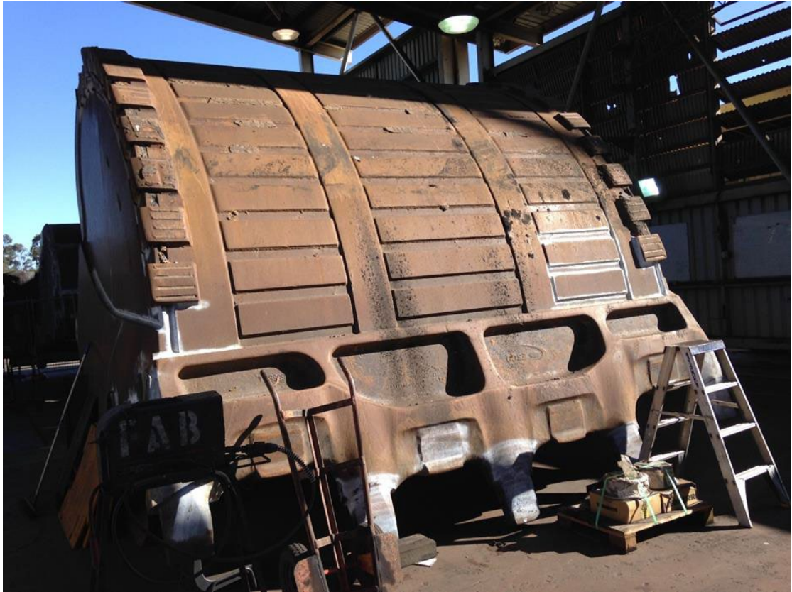
[OEM] Original wear package – smaller horizontal plates
