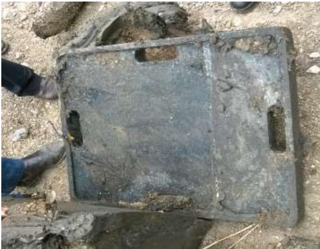
Figure 7: View of the recovered stabiliser pad upon which the rear passenger’s side outrigger leg was placed. Note the soft underground of clay below the hard gravel crust.
