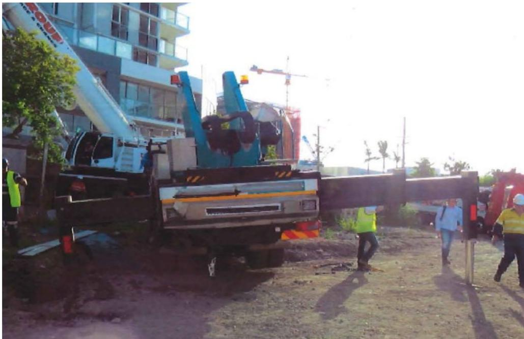
Figure 5 – The subject EWP after being recovered and “uprighted” but not returned to its original position. Note the rear outrigger “arm” on the passenger’s side is not fully deployed to 3 metres unlike the driver’s side leg. It was half deployed at 1.4 metres which reduced the “spread” of the load.
