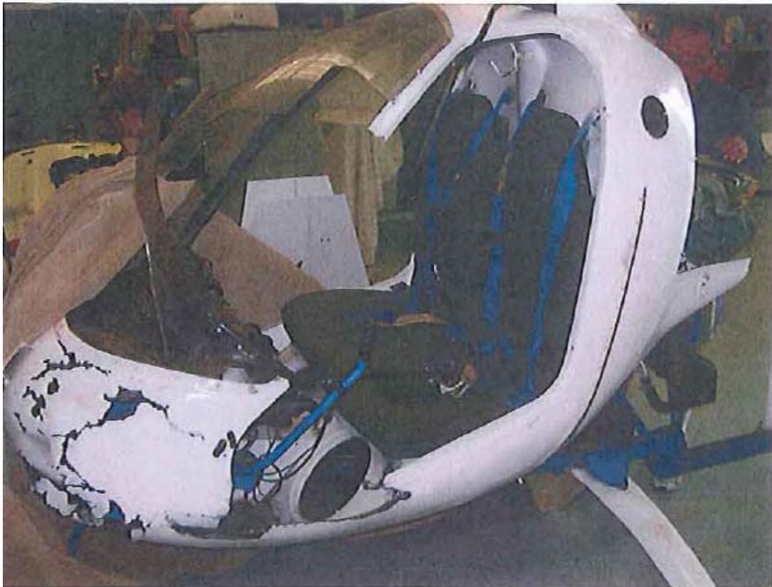
Photograph 1. Front damage to the body of the Gyrocopter.
