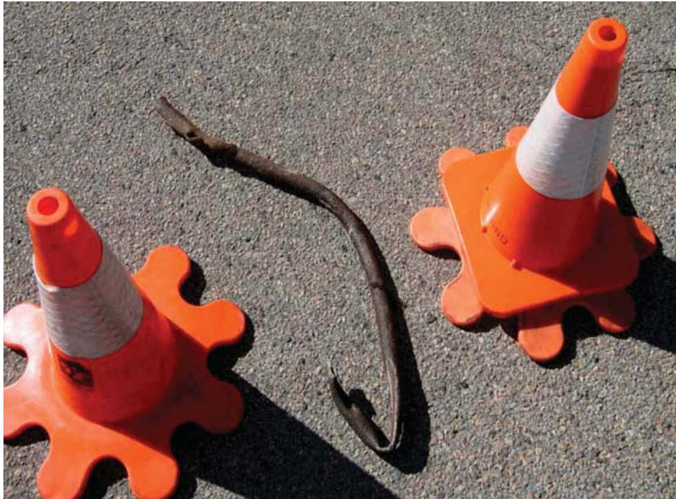
Photograph showing the section of metal pipe found on the road
