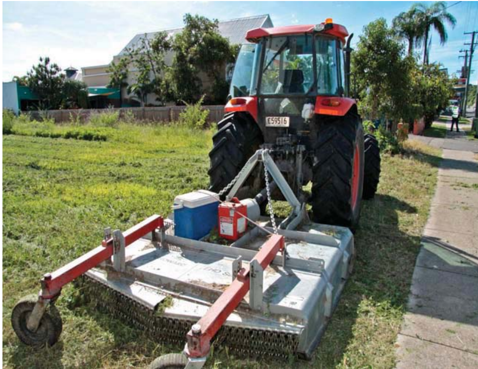
Photograph of tractor and slasher – a curtain of chains across the rear opening of the slasher
