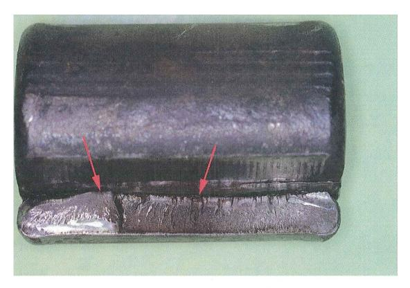
Fatigue fractures the main spring had initiated at the locations arrowed.
